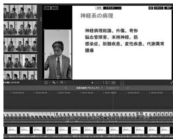
Figure 3. Record the screen of the computer and the teacher's appearance, then combine both images into a single video based on the audio recording
